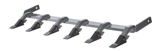
Our bolt-on tooth bar slides over the cutting edge and bolts to the side of your bucket. Easily remove the tooth bar from your bucket by simply removing two bolts. These are built to fit our standard size buckets, however, we can custom build for any size bucket.
